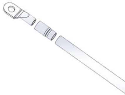
Figure 3-15 Copper terminal, heat shrink tube and copper wire.
