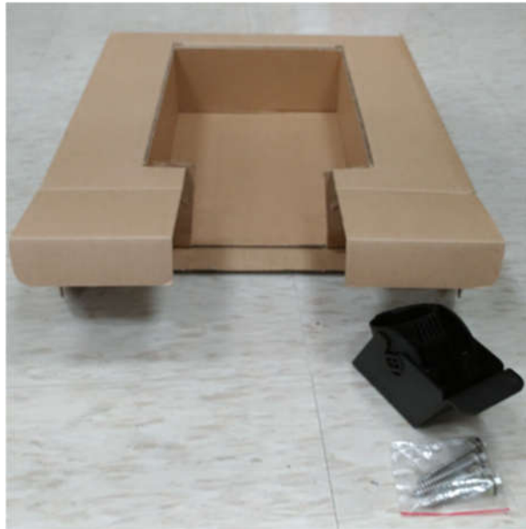
Figure 1-7 Accessories inside the middle partition
