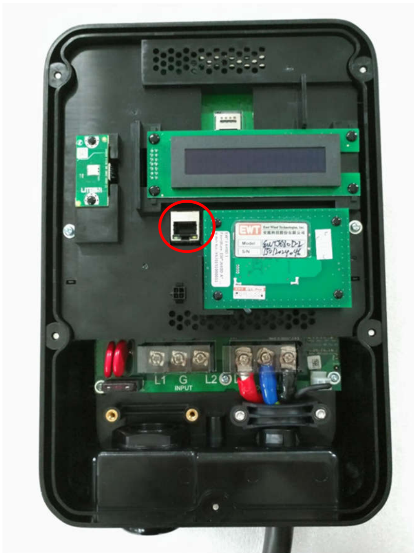
Figure 3-24 Location of Ethernet RJ-45 port
